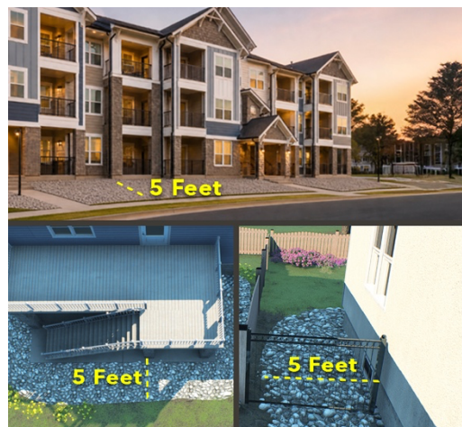
Figure 2. The 0-5 Foot Noncombustible Zone
