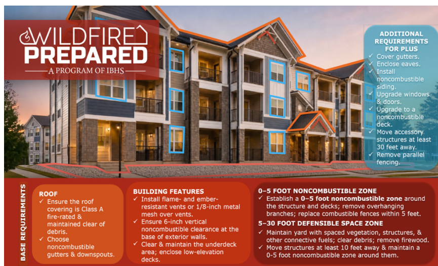
Figure 1. Abbreviated List of Requirements
